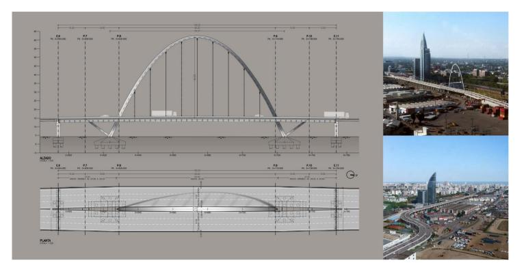
The Montevideo Harbor Access Improvement Project comprises two access ramps each 200 meters long, a 1,800 m long precast cornet viaduct 8 m above ground level, and an arch bridge 160 meters long to be located beside the Montevideo Central Station. The viaduct will be 24 meters wide, and will have three lanes in each direction. The actual roadway in the ground level has two lanes per direction.
